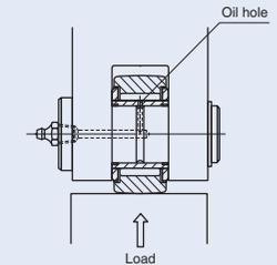
Fig. 2 Position of oil hole and load direction
