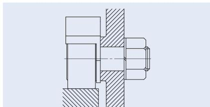
Fig. 7 Mounting of C-Lube Unit
