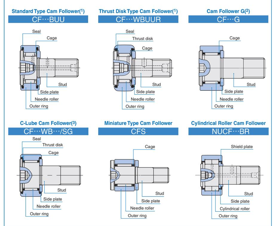
Note<sup>(1)</sup> In case of the stud diameter ( $d_1$ ) 5 to 10mm, a re-greasing fitting is provided in the stud head hex hole. The stud diameter ( $d_1$ ) 12 to 30mm, a grease nipple is provided in the stud head hex hole.
